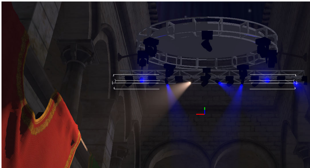
Cycle through the selected conventional fixtures to focus them one at a time; the fixture to focus is highlighted
